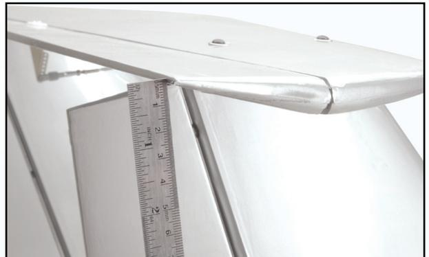
Rudder: 60mm each way at base of rudder, with no exponential
