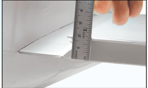
Elevator: 27mm each way at tip of elevator, with 20% exponential
