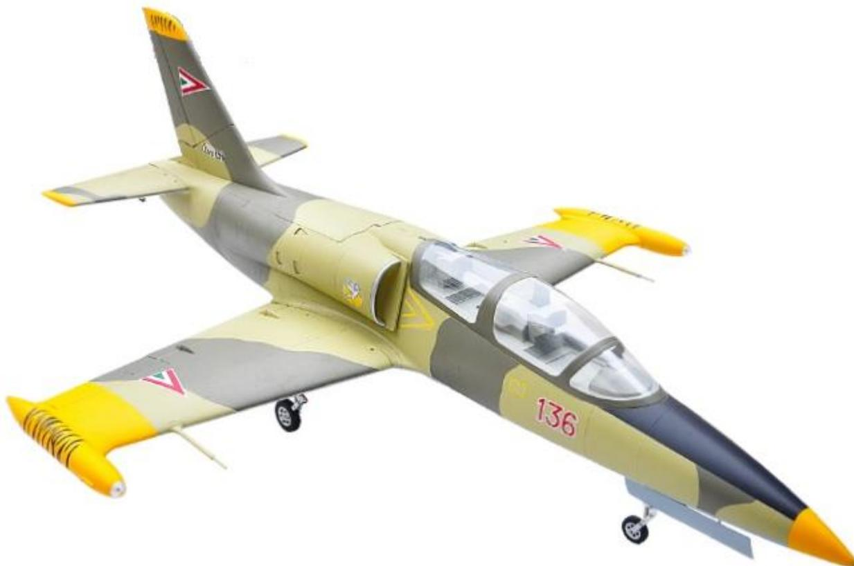
CG 115 mm (4.5 inches) from leading edge at root of wing to fuselage.
