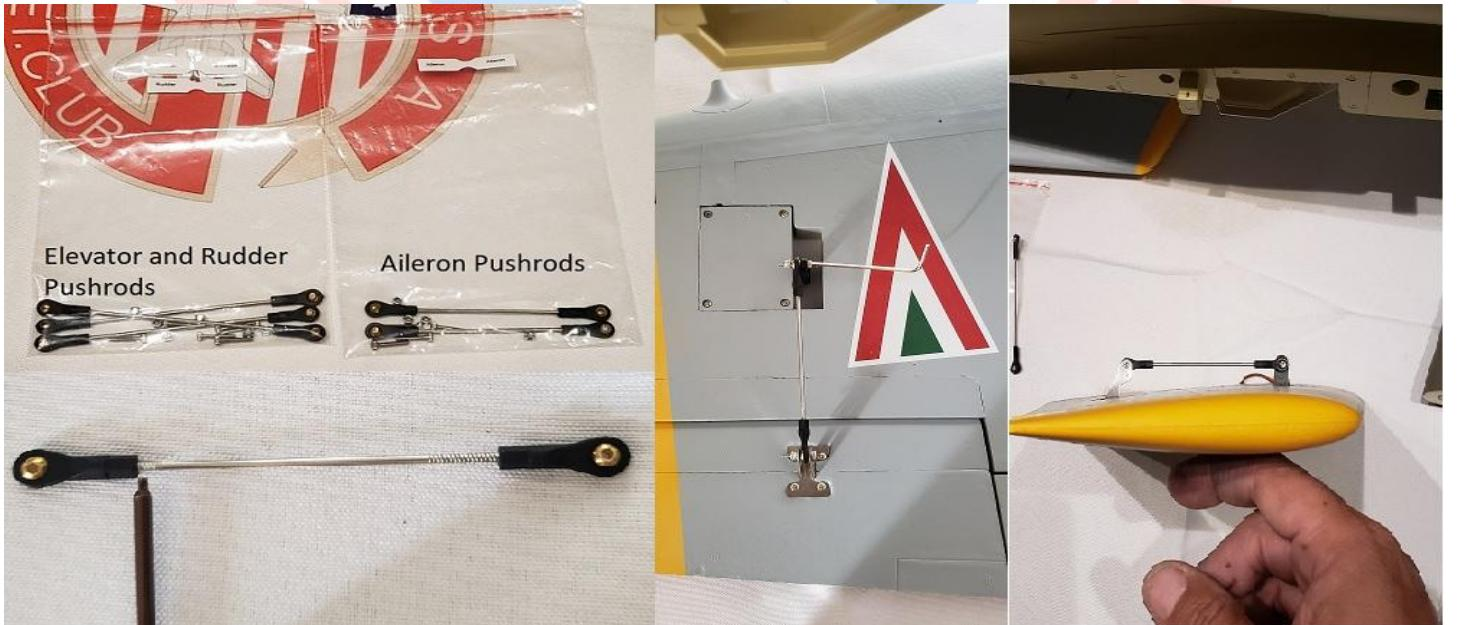
**RUDDER:** On the Elevators, Rudder and Ailerons, you want to center the servos and then install your pushrod so that the servo arm and the control horn are 90 degrees to the flying surface like in the picture of the Elevator. On the vertical fin there is a scale baffle the you will have to glue to the top of the Fin right on at the top of the rudder. Use your favorite glue, if you use CyA, try to use a Foam Safe type of your favorite brand. Alternative, you can use Epoxy.
