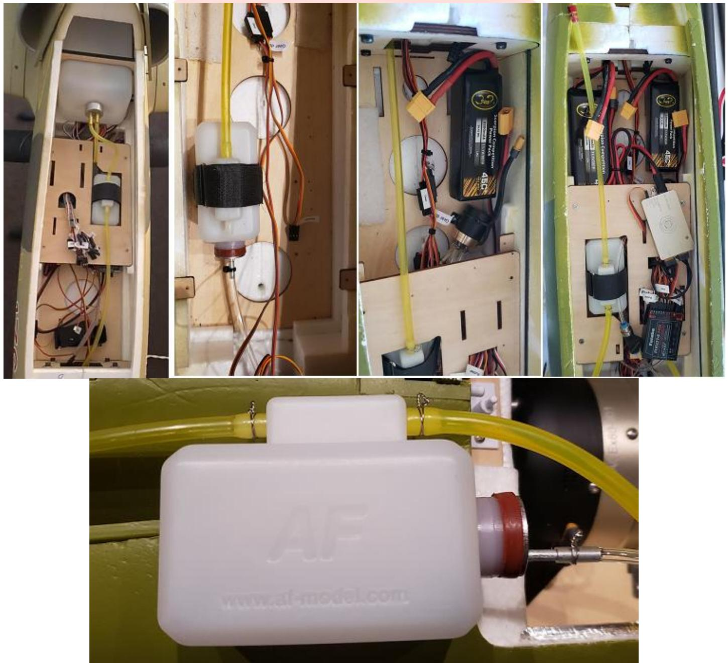
**Turbine Installation:** If you purchased one of our ACEx60 or ACEx80 Turbines, then you will see that the mounting holes have already been drilled on the wood Turbine mounts and there is no other guesswork to be done. This will also insure that you have a gap of 1.5 inches from the rear tailcone of the Turbine to the start of the actual pipe. This gap should not be confused with the start of the aluminum bell mouth.
