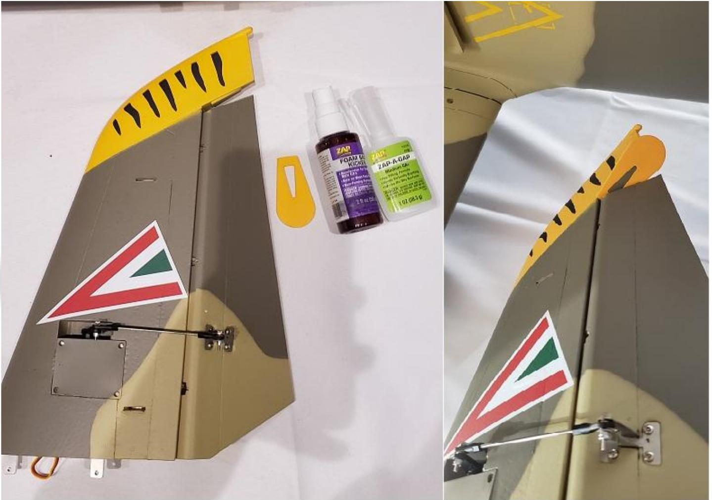
**FLAPS:** The servo for the flaps, in the UP position, you will have the servo arm at about 45 Degrees at neutral. Adjust the pushrod as needed and install Again, use the hole in the servo arm that is closest to the servo and the top hole in the Control Horn in the Flap. This will give you more control in the entire range of motion instead of having to limit the amount of travel in your flap channel later.
