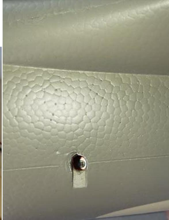
When installing or removing the fan, you will have to install the two screws from the top of the fuselage, you might have to look through the top to make sure to align your screwdriver with the screw deep in the fuselage. If you are removing a fan, it is best to first carefully remove the plastic air diverters from the front of the fan, thus allowing you to see the mounting screws better and provide a different angle to view the fan mounts.
