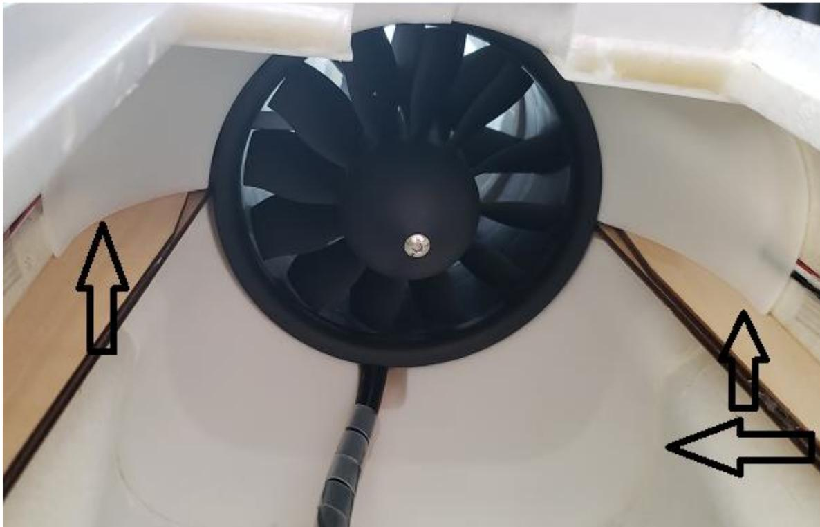
The below installation shows a JP Fan with the two plastics diverters removed. The airframe only has two openings on the top of the fuselage, the plastic diverters hold the fan in place in the front section.
