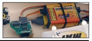
Install the receiver on the right hand equipment plate using double sided tape and neaten the wiring using cable ties.
