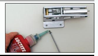
Test fit the main undercarrage and pre-drill the mounting holes. Use a felt tip pen to mark the sides of the recess where the air line holes are needed.
