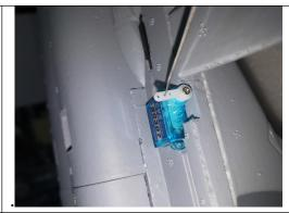
(4)Power on servos and make the arms centered, and then assemble the push rod of horizontal tail.
