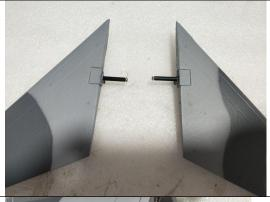
(2) Taking out screws of Horizontal tail plugs. Then assembling horizontal tail into fuselage, finally fixing with screws.
