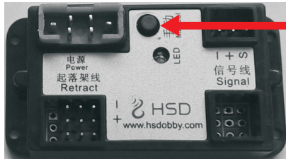
Manual switch for landing gear 'Up/Down'.
