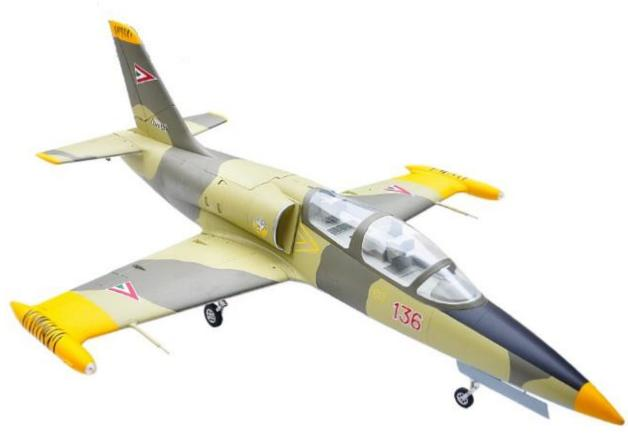
CG 115 mm (4.5 inches) from leading edge at root of wing to fuselage.
