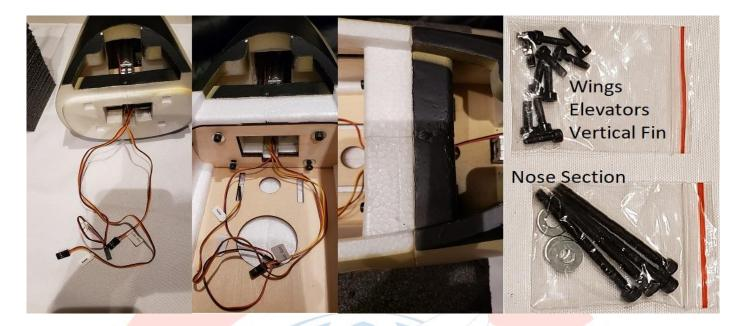
**Nose section:** There are three servo leads coming out of the nose section, make sure you pass them through to the fuselage. Find the 4 Metric 4x50 (two inches long) screws and washers. You will need to insert those through the main fuselage into the nose section. You only need to make them snug enough until all the gap on the side of the fuselage is gone. Do not over tighten and crush the foam.
