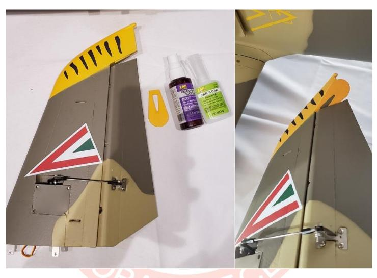
**FLAPS:** The servo for the flaps, in the UP position, you will have the servo arm at about 45 Degrees at neutral. Adjust the pushrod as needed and install Again, <u>use the hole in the servo arm that is closest to the servo and the top hole in the Control Horn in the Flap. This will give you more control in the entire range of motion instead of having to limit the amount of travel in your flap channel later.</u>
