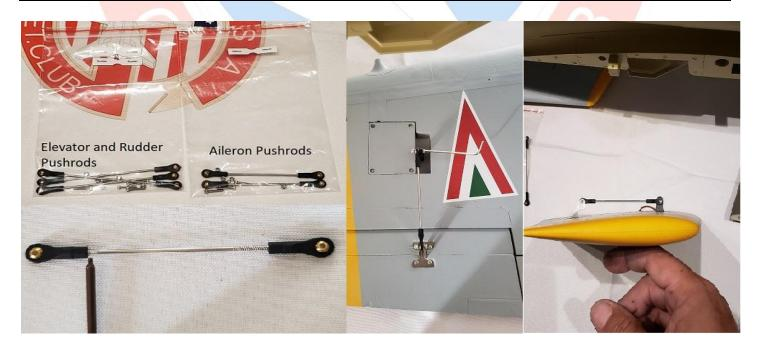
**RUDDER:** On the Elevators, Rudder and Ailerons, you want to center the servos and then install your pushrod so that the servo arm and the control horn are 90 degrees to the flying surface like in the picture of the Elevator. On the vertical fin there is a scale baffle the you will have to glue to the top of the Fin right on at the top of the rudder. Use your favorite glue, if you use CyA, try to use a Foam Safe type of your favorite brand. Alternative, you can use Epoxy.
