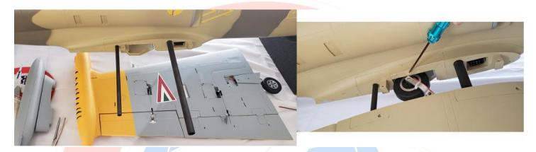
**ELEVATORS:** Find the elevator spar which is about 19.5 inches, feed the spar through the fuselage and then install each elevator half making sure to connect the servo extension on each side first, then use two Metric 3x10 screws to hold the elevator into the fuselage.
