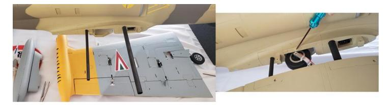
**ELEVATORS:** Find the elevator spar which is about 19.5 inches, feed the spar through the fuselage and then install each elevator half making sure to connect the servo extension on each side first, then use two Metric 3x10 screws to hold the elevator into the fuselage.
