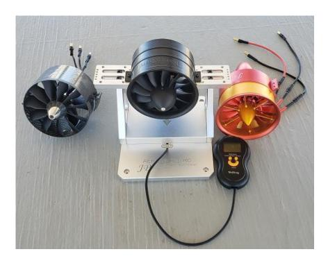
The EDF is partially supported by three plastic air diverters that route the air to the center of the airframe. If you purchased one with a fan already installed, you would need to carefully remove the top two diverters should you need to remove the fan for any reason.
