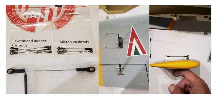
Control Throws: Use the lowest hole possible on the servo arm and the highest hole on the control surface. Since the required travel is very small on all, but the rudder on all of our flying surfaces, in order to get the best resolution / control from your radio, adjust the surfaces to your liking, we recommend settings that will give you more control over the entire range.
