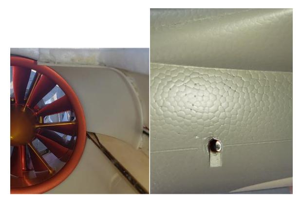
When installting or removing the fan, you will have to install the two screws from the top of the fuselage, you might have to look through the top to amke sure to align your screwdriver with the screw deep in the fuselage. If you are removing a fan, it is best to first carefully remove the plastic air diverters from the front of the fan, thus allowing you to see the mouting screws better and provide a different agle to view the fan mounts.
