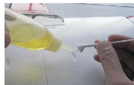
7. Instale as antenas com cola.
