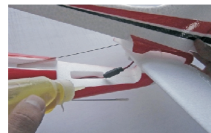
10 - Apply glue to the tail, and then glue it to the fuselage.
