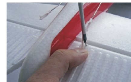
11 - Fix the control rods with screw.
