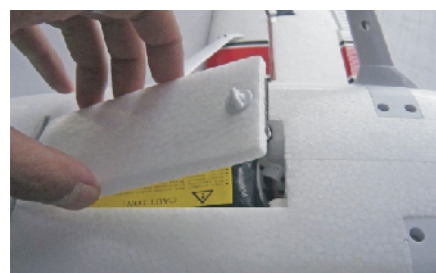
19 - Lock the battery apartment by switch.
