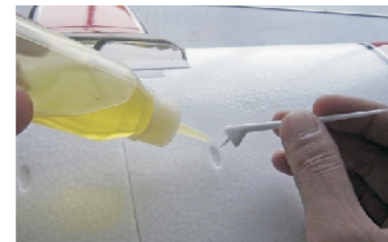
7 - Install the antennas by glue.
