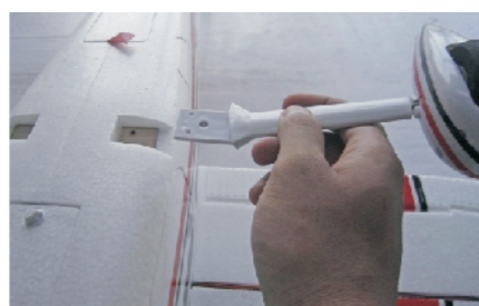
14 - Insert the main landing gear to the fixed seat on both sides of the fuselage.
