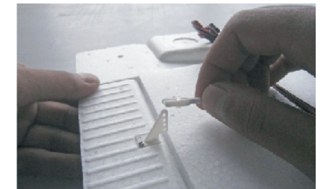
3 - Fix the clevis by hand (The first hole).
